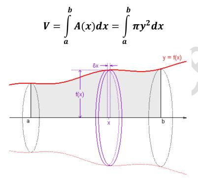
Example:- Find the Volume generated by rotating the bounded area by  $y = x^2$  and the line x = 4 about x-axis
